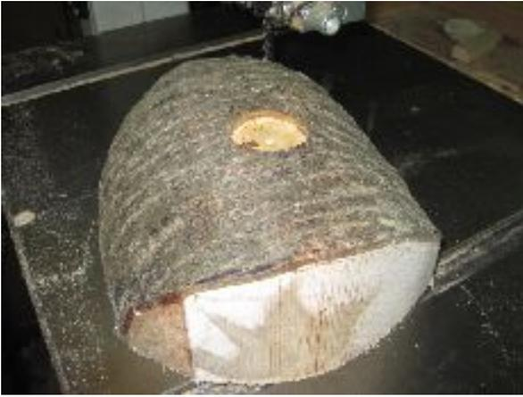
I've cut my blank on the bandsaw and drilled a 1 3/8" hole through the bark into the more solid sapwood in the center of the blank to give me a good, safe seat for my spur center.
