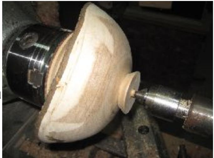
Finally I turn away the all but the last bit of the bottom of the foot leaving a small nub that I'll carve off after it's off the lathe. I generally sand the foot, neck and the transition area of the bottom of the bowl at this time but the remainder of the sanding will take place off the lathe.
