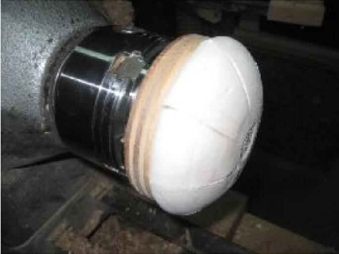
To finish the pedestal foot I'll be reversing the piece onto a jam chuck I made from some plywood and walnut. The jam chuck has a gently curved face covered with self-adhesive foam bought at a local craft store. I'll place the bowl over this and bring up the tailstock to "jam" it into place.
