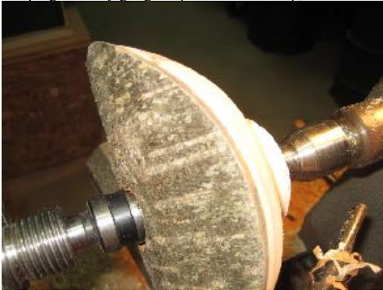
You'll note how crisp the bark edge is in this photo as a result of cutting carefully in the "wrong" direction. This is where the higher speeds help, giving your tool less time in mid air and more time in contact with the wood. Be careful and always watch the "ghost" image that the spinning piece shows. If you have trouble seeing this try taping a sheet of light colored cardboard across the bed of the lathe. The contrast may allow you to see what you're cutting better.
