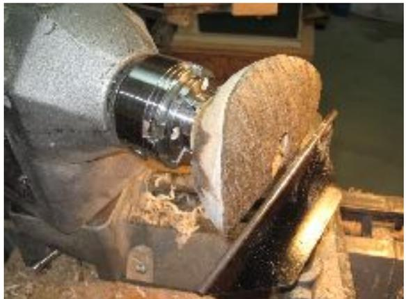
Next, we'll begin the process of removing material from the inside. Natural edge bowls require a little more care than a typical green wood turning as the height of the edge is variable and will begin warping as soon as we start removing material from stress release, moisture loss and tool pressure on the un-supported wings as well as centrifugal force.
