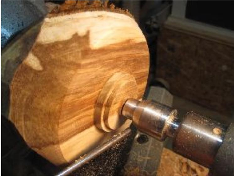
The step illustrated here serves a dual purpose. The smaller diameter tenon is what I'll actually grip the piece with in my scroll chuck. The larger diameter serves as a seat for the top of the chuck's jaws. This section will eventually get turned away and form the "neck" of the pedestal foot.
