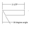
Adjustable stop and fixed stop are both ¾ poplar. The steps are cut in 1" increments.
