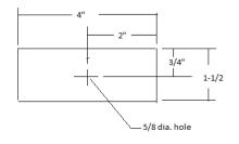
Yoke support (part E) make 2 Round top front corner for clearance Middle block (part C) 5/8 hole thru middle of used 1 ½ baluster stock for this piece.
