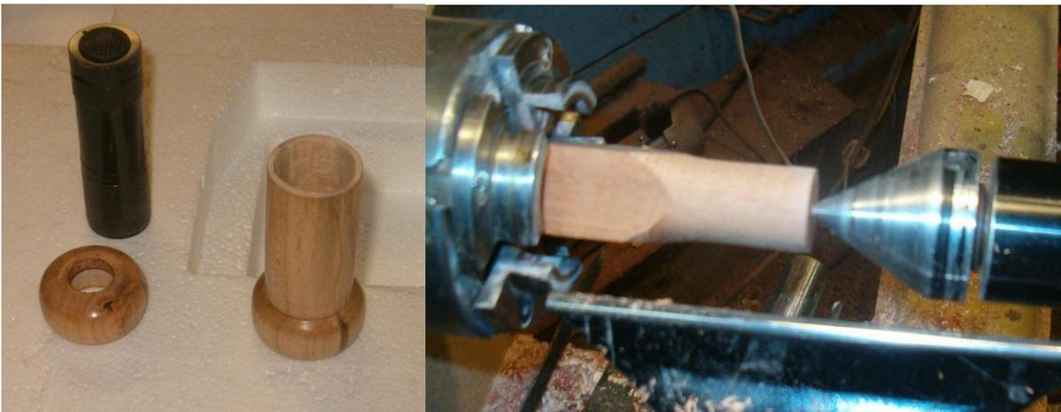
The cylinder is now completed, except for the button. This can be made from the remaining part of the cylinder or a contrasting wood. I usually use a piece of wood 1" square turn down to a 7/8" dia.
