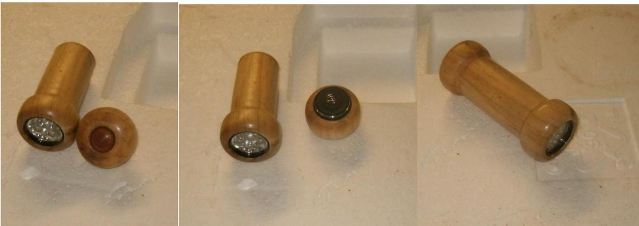
Slide the flashlight into the main sleeve and apply a couple of drops of medium CA near the lens end of the flashlight to hold it in place. Put a couple of drops of CA on the sides of the flashlight cap and install the turned top. Line up the grain between the two pieces. And don't forget to put the button in. The cap can be screwed off to change the batteries.
