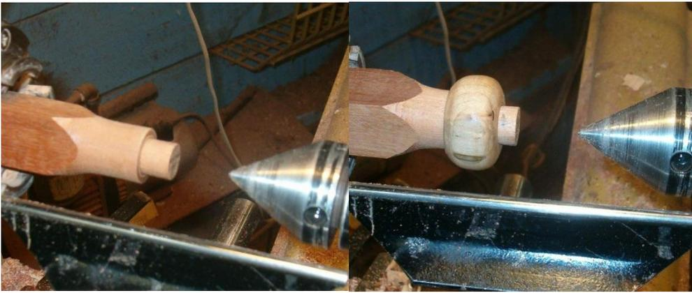
Turn a tenon just under 5/8" dia. About 3/4" long. Use the cap to make sure the piece is a loose fit, and to mark the finished length of the button. Trim the tenon to length, sand and finish.
