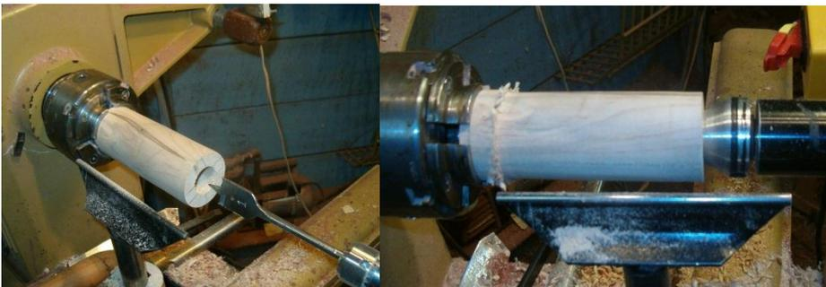
Mount the cylinder in a chuck, and drill to a depth of 3". Check to make sure the flashlight slides into the cylinder. If not, sand the inside for a smooth fit. Bring up the tailstock and retrue the cylinder if needed.
