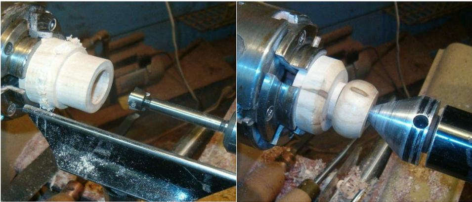
True up the face of the remaining section and bore with a 1" forstner bit to a depth of 5/8". Then bore a 5/8" hole
