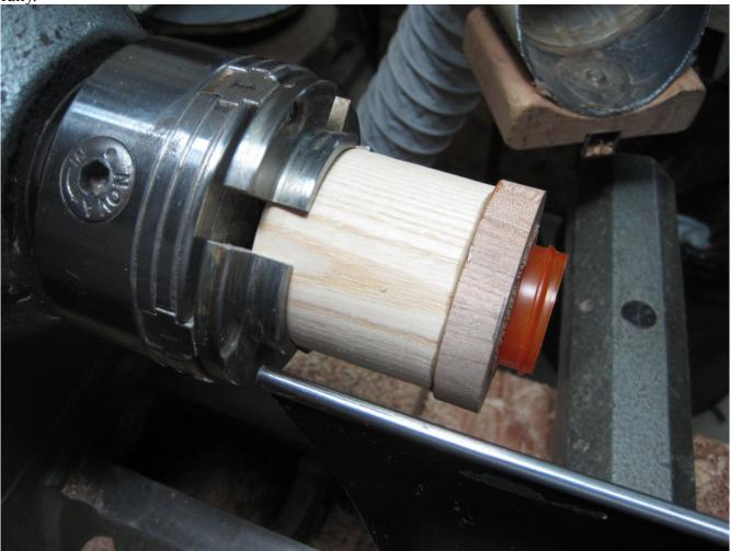
When fully cured, screw the cap assembly onto the body/ring assembly. Place the open end of the bottle body end over the tenon of your base (that's still in the chuck) and snug up with your tailstock.
