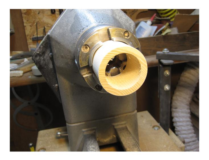
Part this section off to give you a hollow wooden tube. (I find it's more useful to part it NEARLY off then finish with a saw to reduce the splintering that parting into a hollow can yield.)
