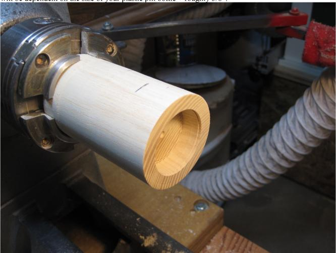
True the end of your blank making sure it's flat across (no convexity or concavity) and, using the proper sized Forstner bit, bore a hole in the end of the blank the same depth as the cap + roughly 1/16 of an inch. Enlarge as necessary to ensure a snug (but not necessarily forced) fit.
