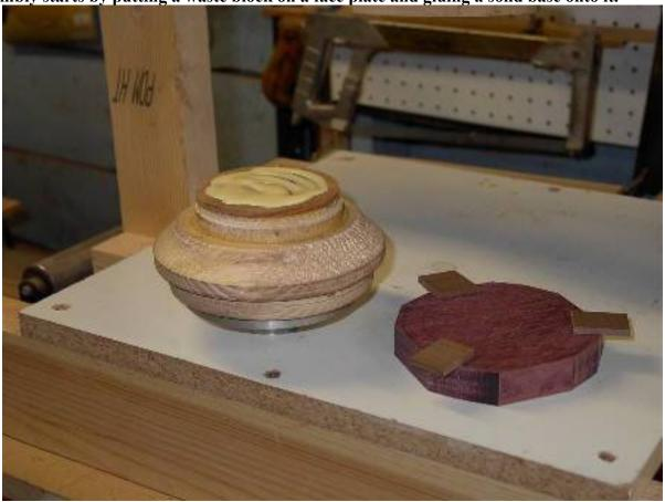
I use scraps hot glued around the rings to maintain alignment.
