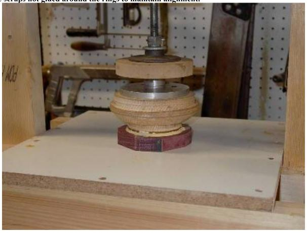
Rings are then added one at a time, aligning to the previous one in a brick pattern for strength. They are put in the press for a min of 30 minutes.
