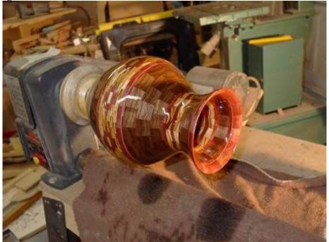
The top coat is two coats of Johnson's paste wax buffed in on the lathe.
