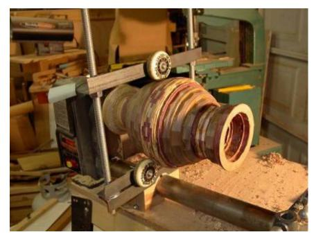
Shaped the inside of the neck to allow a plug to be inserted and the tail stock to be used.
