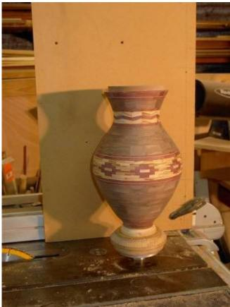
The outside is then finish shaped with bowl gouges and scrapers.
