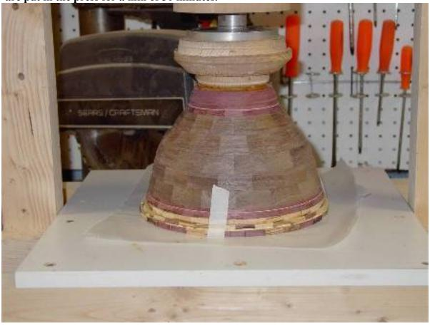
As each layer is added it is trued on the lathe and the segment corners are knocked of to help
