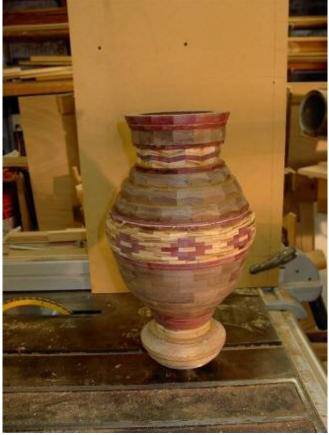
Due to its size this piece was unstable even at slow speed. I set up the steady rest at the largest point
