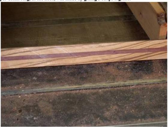
Then cutting at a 30 degree angle, and gluing into pairs.
