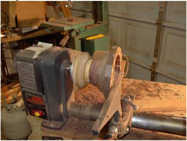
The large detail ring was an easy one on this project. Just time consuming; it contained 224 pieces in 7 rings. Layered as described before.
