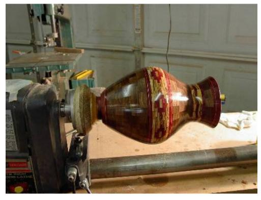
The next step is the scariest, after almost 6 weeks and 150 hours of work, parting off the piece and finishing the base. I reverse mount the turning between a jam chuck and tailstock, then
